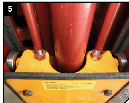
▲ Each carriage rolls on (8) 4" double sealed, self lubricating, heavy duty ball bearing rollers for a lifetime of trouble-free service (not plastic slide blocks).
