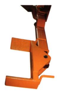
Using the wheel engaging adaptors on your MOHAWK LIFTS makes vehicle set-up quick and easy. Especially for vehicles with hard to reach frames.
