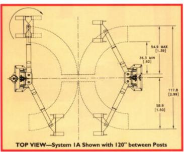
MODEL WA-I capacity is 6,000 lbs. (1500 lbs. per arm) designed for MOHAWK SYSTEM I LIFTS.
